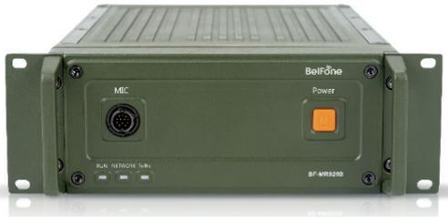
MESH base stations are mainly deployed at fixed points. The equipment has high transmission power and long coverage distance. It is especially suitable for scenarios such as long-distance coverage communication, information convergence and return, regional coverage support, commanding coverage, and repeater transmission nodes.
